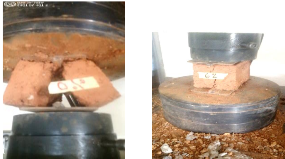
Figure 5. Failure Mode of The Specimens Under a Tensile Loading. (a) Control Specimen; (b) Reinforced Specimen
